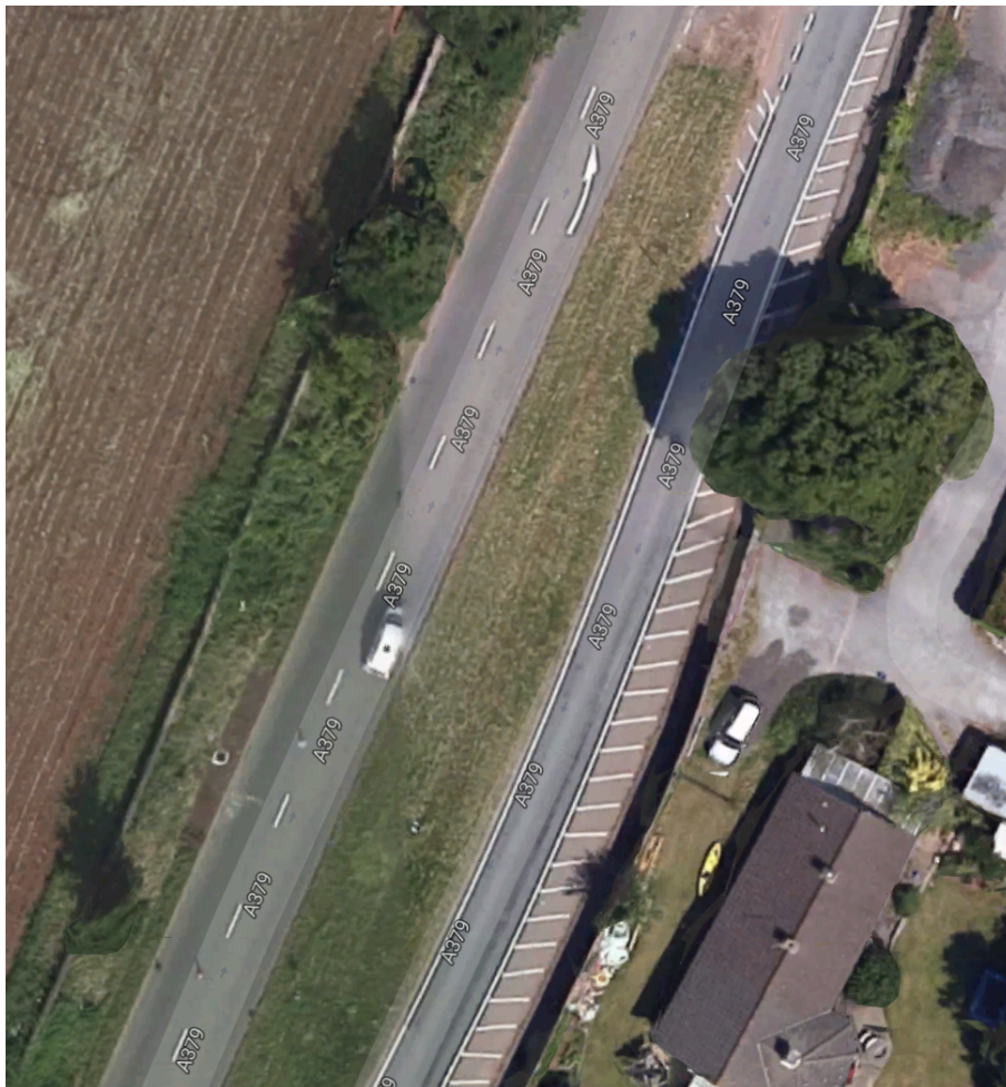
Image 3 – Design example of segregated infrastructure for vehicles, cycles and pedestrians. Note that widths are suitable for one way cycling – this design would need to be replicated on both sides of the street to be effective. Image credit to Sustrans.
