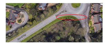
The A379 overbridge currently has only paint on the road to demarcate the path for cyclists and motorised vehicles. If this bridge is to be used by both buses then there needs to be some protection physical for people cycling.
