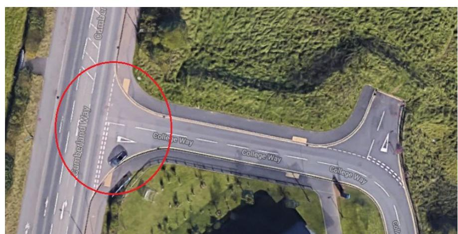
this junction should be tightened and priority given to these active travellers. This can be achieved with a raised table, coloured tarmac and give way priority changes.
