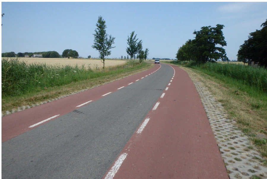
Fig 2. Designated cycle paths which prioritise people cycling. Cars need to pass (this design is only acceptable in a very lightly-trafficked road).
