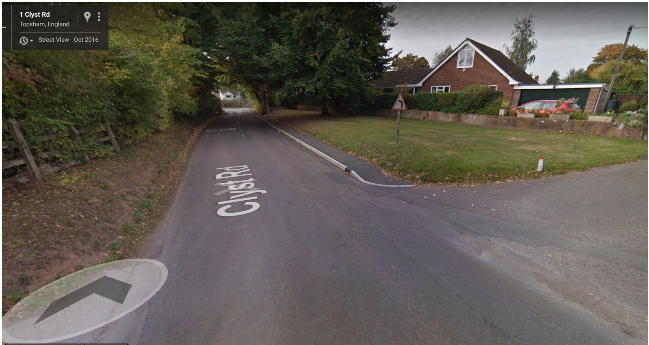
Figure A: Looking south down Clyst Road towards Topsham. The proposed 2m footway will link to the narrow pavement to the right. A minimum 3m wide path must be provided along the full length of Clyst Road.
