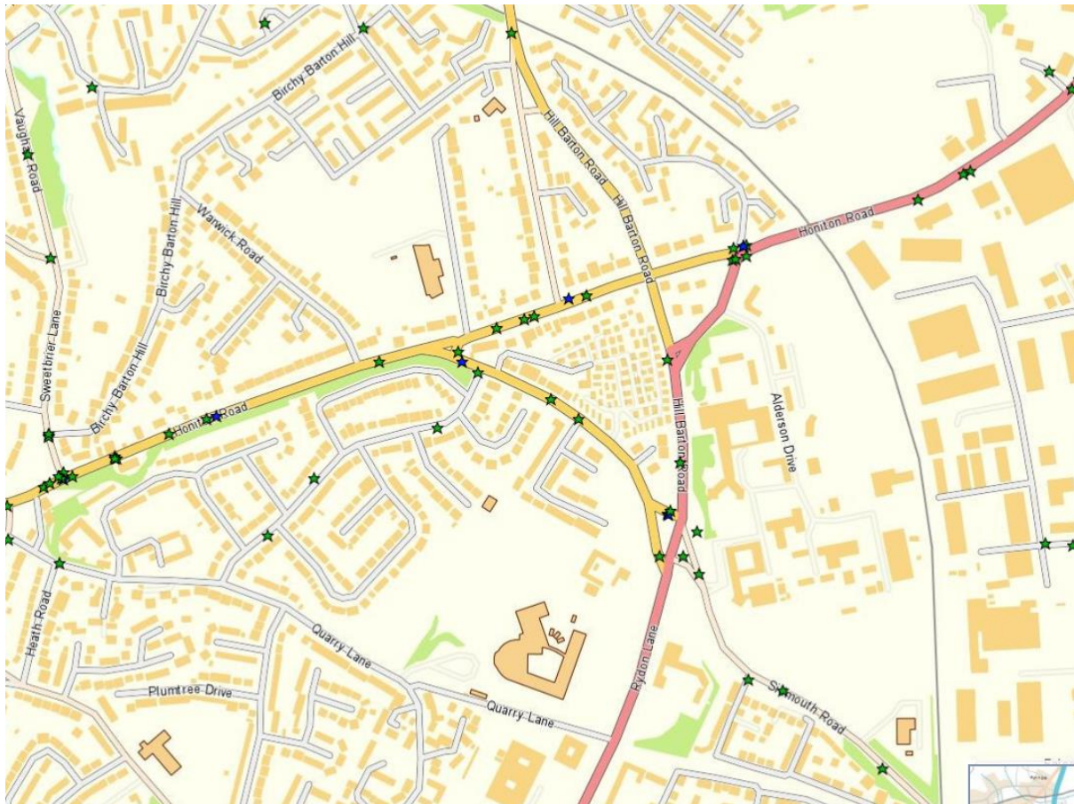
Figure 1: Devon Collision Map, showing numerous collisions along Honiton Road with high numbers of collisions in the immediate vicinity of the proposed development.
